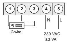
Type M1-1VR4B.0001.770xD with a supply of 24 VDC, galv. isolated
