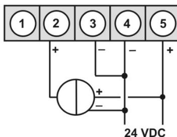
**M1 in combination with a 3-wire-sensor 0-10 V**
