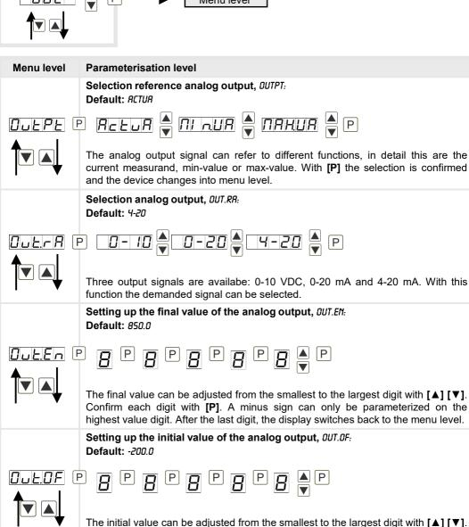
Confirm each digit with [P]. A minus sign can only be parameterized on the highest value digit. After the last digit, the display switches back to the menu level.
