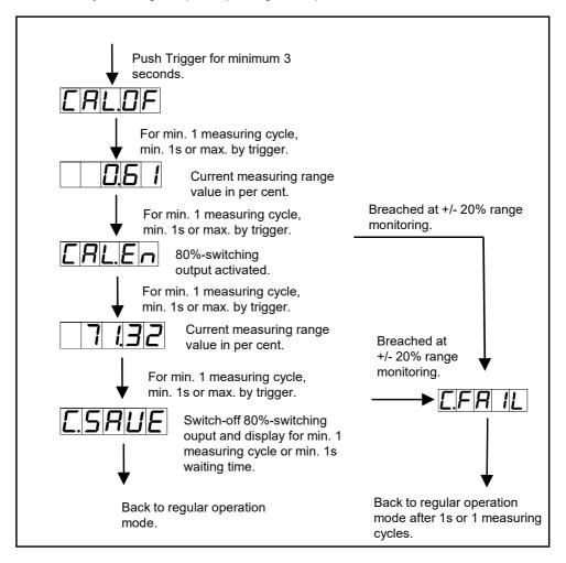
If a special input range *SEN5.1*, *SEN5.2*, *SEN5.3* was selected under *TYPE*, a checking of the range is done for offset and final value. At an undercut/exceedance of  $\pm$  20% of adjustment range, an *C.FRIL* is given out.
