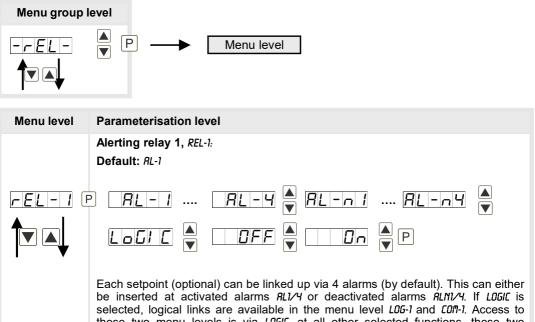
these two menu levels is via *LOGIC*, at all other selected functions, these two parameters are overleaped. Via *DN/DFF* the setpoints can be activated/deactivated, in this case the output and the setpoint display are set/not set on the front of the device. With **[P]** the selection is confirmed and the device changes into menu level.
