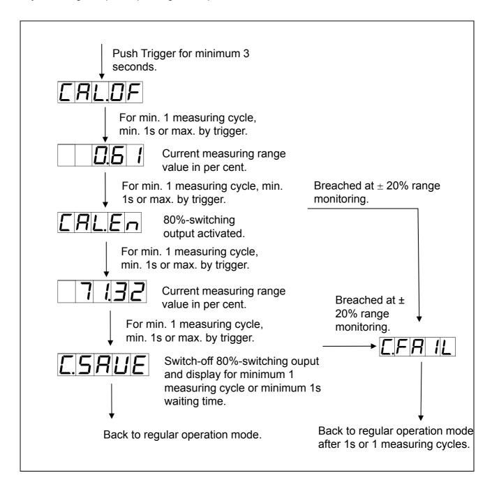
If a special input range **SENS.1**, **SENS.2**, **SENS.3** was selected under **TYPE**, a checking of the range is done for offset and final value. At an undercut/exceedance of  $\pm$  20% of adjustment range, an **C.FRIL** is given out.
