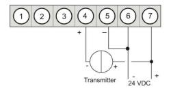
M3 in combination with a 3-wire-sensor 0-10 V
