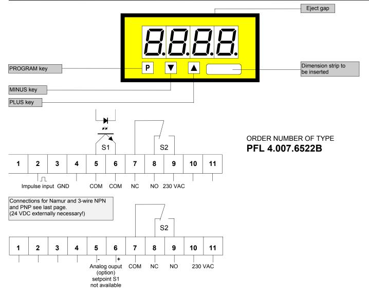
Power supply 115 VAC (connection via terminal 10 and 11)
