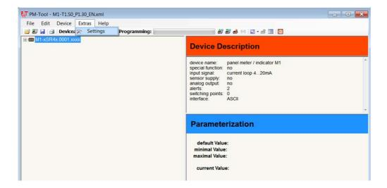
Via a check box available COM addresses can be selected. A standard PC comes in general with two COM interfaces. Using a laptop, generally a USB-RS232 Gateway is used. The driver of the gateway simulates a RS232 interface, so that a COM-Port feely assigned and runs with this software, too.
