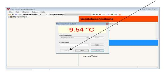
For further processing the current measurand can be filed under a csv file on the PC and with a machining program for visualization be represented as e.g. a data logger.
