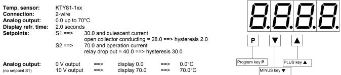
The basic adjustments concerning to the following program example are the ground parameters after a total reset occuring through a power on with pressing **P**-key (see previous page).
