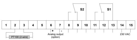
Power supply 115 VAC (connection via terminal 14 and 15)
