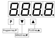
The basic adjustments concerning to the following program example are the ground parameters after a total reset occuring through a power on with pressing **P**-key (see previous page).
