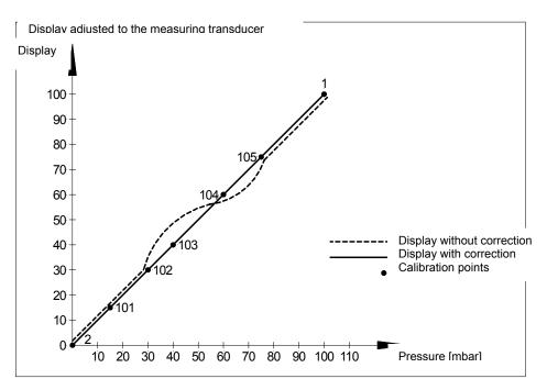
Linearisation of a pressure transducer for 0...100 mbar with a sensor of 2 mV/V.
