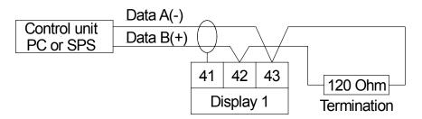
**Caution!** The potential reference can lead to a compensating current (interface ⇔ measuring input) with a non-galvanically insulated interface and can thus affect the measuring signals.
