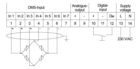
Measurement of a **4-wire sensor** with a **PM5** with an actively switched digital input; auxiliary voltage 24 VDC
